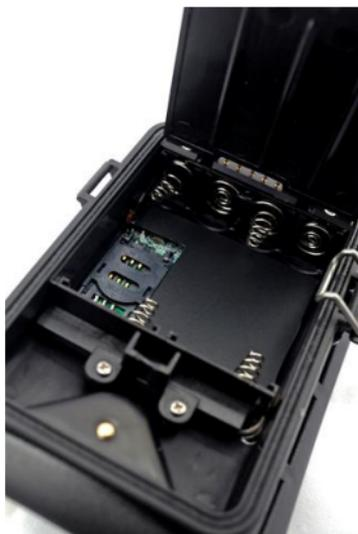
Figure 2-1 MMS-module Battery Box
